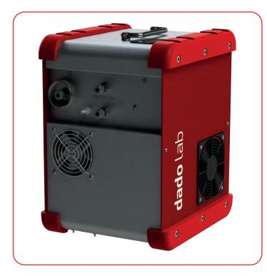
The sample suction pump was specifically selected to grant high compensation to ensure an operative flowrate of about 2 l/min and high pressure drop compensation.
